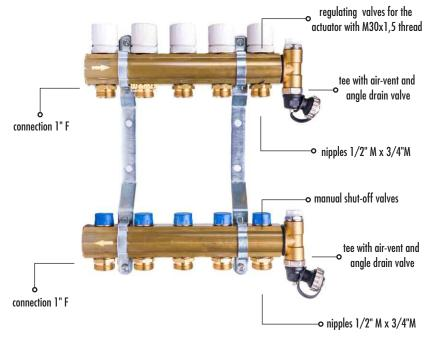
Brass manifolds **CM-NRT** are used to separate individual loops of floor heating and their proper regulation, ensuring comfort of use and even distribution of heat. It contains two C-profile beams connected with two steel holders, connections for supply and return of the system, nipples with an o-ring, manual shut-off valves, regulating valves for actuators with M30x1,5 thread, two brass tees with o-ring, manual air vent and angle drain valve.
